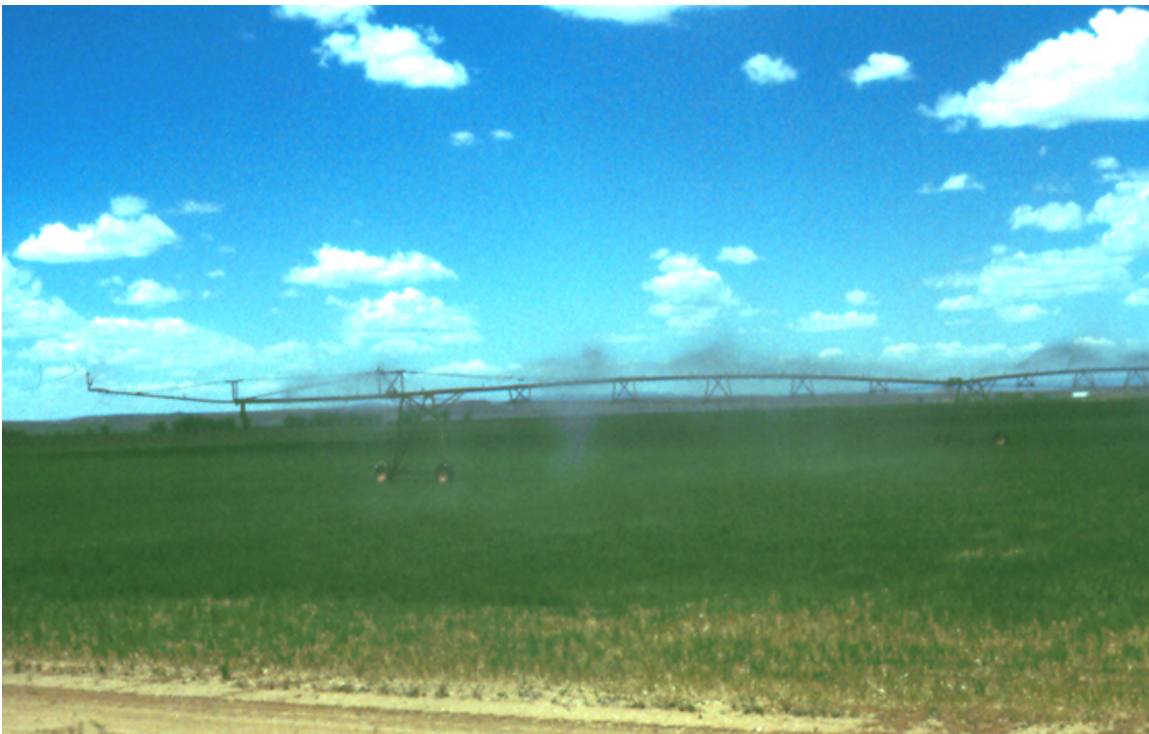
FIGURE 8: Center pivot irrigation pipe spraying water on an alfalfa field.
